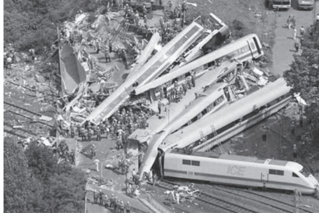
Figure 2. High-speed “ICE” train in Eschede, Germany in 1998. This accident was caused by a crack in the wheel caused by fatigue
