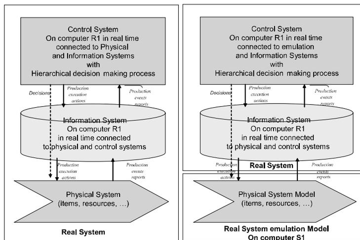
**Figure 1.14.** Emulation system connected to real control system
