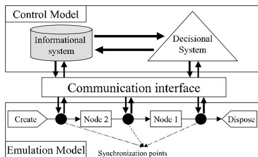
**Figure 1.17.** *Product-driven system simulation*
