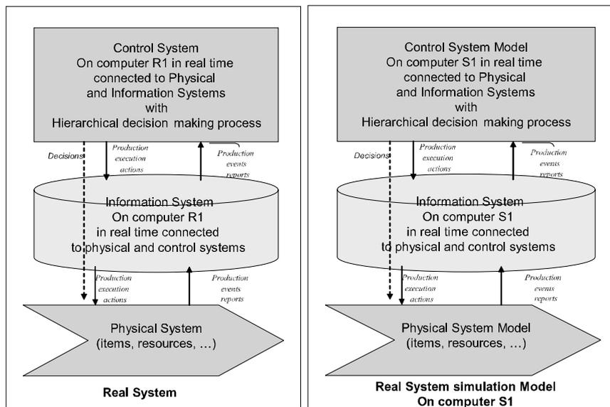
Figure 1.13. Real-time simulation model
