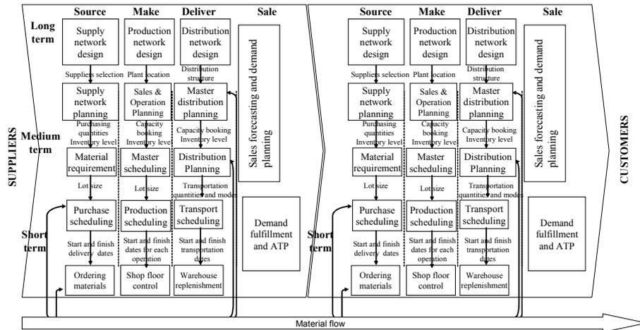
Figure 1.4. Different supply chain decision processes (2 independent units)
